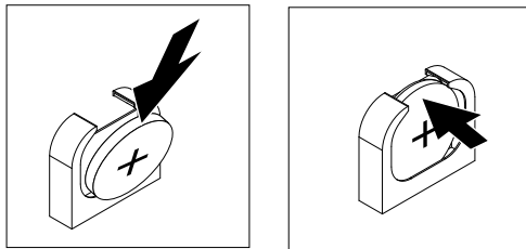
Figure 145. System battery installation
