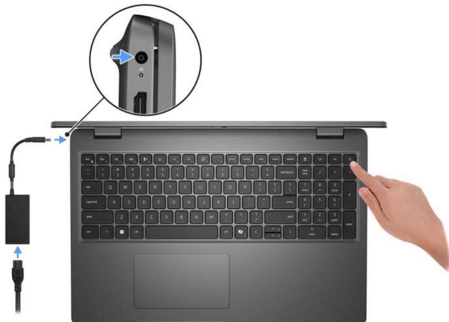
**Figure 1. Connect the power adapter and press the power button.**
