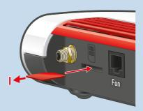
3. Push the SIM card carefully into the SIM card slot with slight pressure until the SIM card clicks into place.
