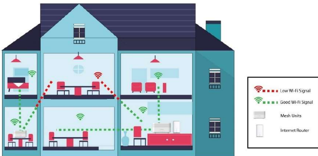
Unoptimized Mesh Installation
